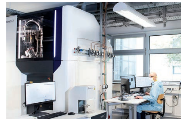
The HT-NAP-XPS system of Fraunhofer ISE provides high measurement performance for material characterization.
